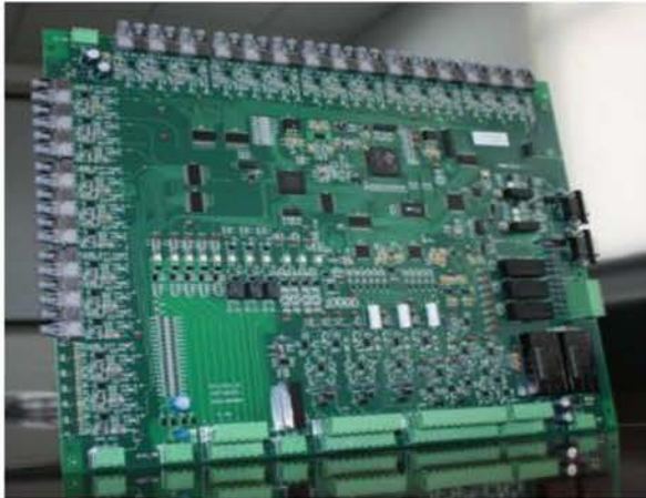
HOFFMANN Single PCB of six-layer
